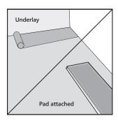
Check to see if there is a pad attached to the back of the panels.
