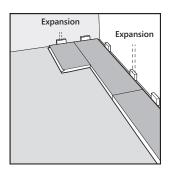
Place the spacers to ensure the correct expansion gap.
