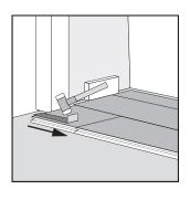
For edge pieces close to the wall, use the pull bar and hammer to completely secure the locking system. Gradually connect the panels in a few taps.
