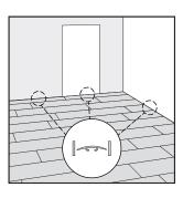
Provide expansion joints between different rooms or in large rooms. Check the supplier's guidelines for details.
