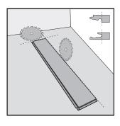
Remove the click profile on every side directly next to the wall to ensure the required expansion gap.
