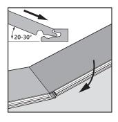
Start on the short side. Position the panel at an angle of 20-30° to the panel that is already installed, and angle down.
