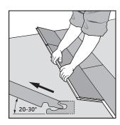
Start by angling out the complete row on the long side of the panel by lifting up to about 20-30°.
