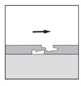
For hard to reach panels, use the tapping method. If possible, angle in one of the sides. Angle down and position the click systems as close as possible.
