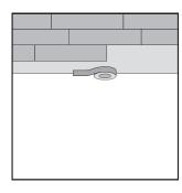
Lay the underlay parallel to the floor direction during installation. Start each new row of underlay upon reaching that point in the floor installation.
