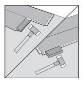
To ensure all gaps are closed, gently tap the tapping block with a hammer to completely close the joints.
