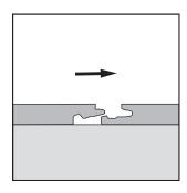
For areas where it is not possible to use angling or a tapping block, such as the end panels against the wall, use the pull bar with the tapping method.
