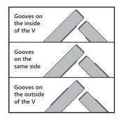
The starting position of the panels is versatile, as long as it's consistent within the rows.
