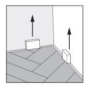
After the floor and expansion profiles are completely installed, remove all spacers from the room(s).
