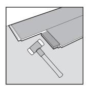
Use a tapping block and position it against the locking system. Gently tap the block with a hammer to gradually connect the panels in a few taps.
