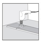
Click the panels together on the short side. Drill a hole centered on the joint between the two panels of the same diameter as the pipe plus 20 mm (3/4").
