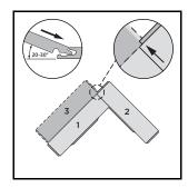
Angle the long side of panel 2 into the short side of panel 1 at 20-30°, slide it towards panel 3 until it reaches the corner of panel 3 and angle down.
