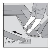
Start by angling out the panel by lifting the corner of the panel to about 20-30° and move the panel fowards and backwards until it releases.
