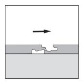
For areas where it is not possible to use angling or a tapping block, such as the end panels against the wall, use the pull bar. Start when the panels are flat on the floor.
