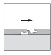
For locking in two sides or if angling is not possible, use the tapping method. If possible, angle in one side of the panel. Tapping is possible on the long and short side.
