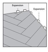
The floor must be able to expand and contract with changes in the indoor climate. For expansion joint guidelines, check the supplier's instructions.
