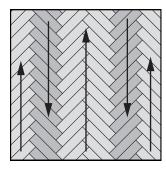
Complete the first V row with complete panels. Make sure to keep it aligned to the center line. Then continue on the sides, working in the opposite direction.
