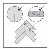
After installing a panel, check all joints to see if they are fully connected and there are no gaps or height differences.
