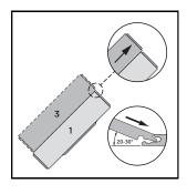
Use an alignment panel (3) to help align panel 2 by installing it 0,5 cm beyond the edge of panel 1.
