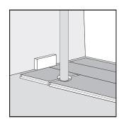
In rows where the flooring meets a pipe, ensure the pipe aligns exactly with the short sides of two panels.
