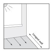
Plan the floor along the longest wall or light direction for the most pleasing visual appeal.
