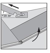
Angle up the end of the panel to angle out the short side.
