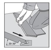
Place your hands close to the joint. Pull the panel towards the installed panels and angle down.
