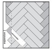
Draw a line by connecting the edges of the installed panels and cut along this line. Rotate the panel back 180° and install it by angling and using the pull bar.
