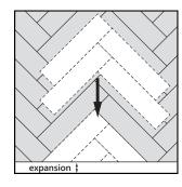
Pre-build the edge pieces with enough panels to cover the gaps. Measure the edges of the remaining floor, taking the expansion gap into account.
