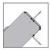
Mark the middle of the short side of the panel. Take this distance and mark it on the long side of the panel.
