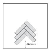
Start the installation at a distance away from the starter wall for easier installation.
