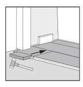
Install the panel on the long side with a tapping block or pull bar. Gently tap with a hammer to gradually connect the panels in a few taps.
