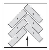
Work in the direction away from the starter wall, with the V pointing away from the wall.
