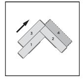
Angle up the long side of panel 3 into the long side of panel 2 at 20-30°, slide it towards panel 4 until it reaches the corner of panel 4 and angle down.
