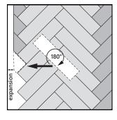
Position the panel in the correct position to be installed. Rotate the panel 180° and position it where it needs to be installed, while leaving space for the expansion gap.
