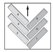
Work in the direction away from the starter wall, with the V pointing towards the wall.
