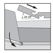
To install the next rows on the tongue sides, angle in the groove under the tongue on the short side, then on the long side.
