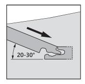
Start on the long side. Position the panel at an angle of 20-30° to the panel that is already installed. Move the panel gently up and down and exert forward pressure.
