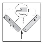
Lay down the panels in the correct start position with the groove side pointing away from the starter wall and to the left side of the V.
