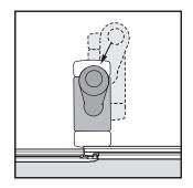
Hammer in the direction of and partly on the underlaying panel. Be careful not to damage the profile or the edges of the panel.
