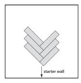
After a few panels, slide the row towards the starter wall, aligned with the center line of the room. Leave enough room for the expansion gaps.
