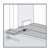
Slide the panel as close to the installed panels as possible. Use a tapping block and a hammer to gradually connect the long sides of the panel in a few taps.
