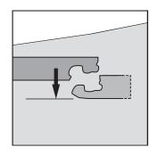
After angling in the long side, drop down the short side of the panel into the short side of the panel that is already installed.
