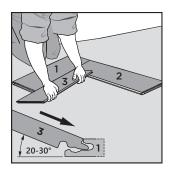
Angle in the long side of panel 3 into the long side of panel 1 at 20-30°, while sliding it close to panel 2.
