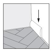
Install skirting on the walls over the expansion gaps to complete the room.
