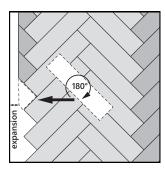
Position the panel in the correct position to be installed. Rotate the panel 180° and position it where it needs to be installed, while leaving space for the expansion gap.
