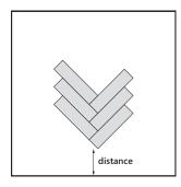
Start the installation a distance away from the starter wall for easier installation.
