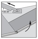
Angle up the end of the panel to angle out the short side.
