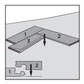
Position the tongue of panel 3 above the groove of panel 2. Press panel 3 down to connect the joints of the short side. Fully connect by hammering down.
