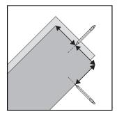
Mark the middle of the short side of the panel. Take this distance and mark it on the long side of the panel.
