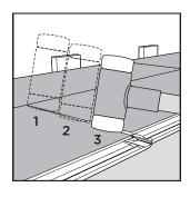
Make sure all joints are fully connected by hammering down on the short sides.
