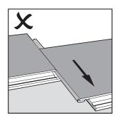
Do not lift up the side of the panel, angle down the edges of the panel, or shift the panels horizontally to disconnect the short sides. Doing so might damage the profile.
