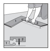
Drop down the panel and fully connect the joints by hammering from the T joint towards the edge of the panel.
