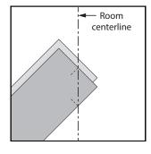
Align the markings on the panel to the center line of the room to ensure the correct angle of the panel and a straight installation.
