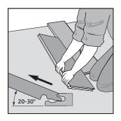
Start by angling out the complete row on the long side of the panel by lifting up to about 20-30°.
