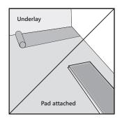
If there is no pad attached to the panels, roll out the underlay in the same direction of the floor.
