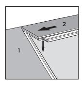
Connect the short side of panel 2 with the long side of panel 1 with a drop down movement.
