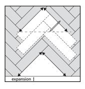
Mark the dimensions on the pre-build panels and cut to size.
