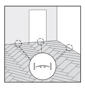
Provide expansion joints between different rooms or in large rooms. Check the supplier's guidelines for details.
