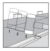
Fully connect the short sides of the panels by hammering from the T joint towards the edge of the panel. Use a tapping block as additional support if necessary.
