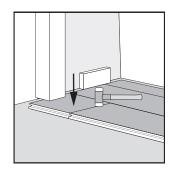
Use a hammer to fully connect the short sides of the panels. Hammer from the T-joint towards the outside of the panel.
