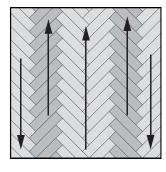
Complete the first V row with complete panels. Make sure to keep it aligned to the center line. Continue on the sides, working in the directions as on the drawing.
