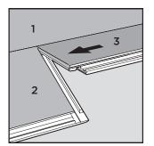
Shift panel 3 to position it so the corner of the head end of the panel is against the head end of panel 2.
