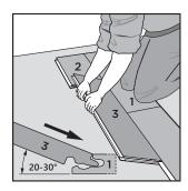
Angle in the long side of panel 3 into the long side of panel 1 at a 20-30° angle.
