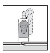
Hammer in the direction of and partly on the underlaying panel. Be careful not to damage the profile or the edges of the panel.
