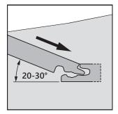
Start on the long side. Position the panel at an angle of 20-30° to the panel that is already installed. Move the panel gently up and down and exert forward pressure.
