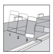
Fully connect the short sides of the panels by hammering from the T-joint towards the edge of the panel. Use a tapping block as additional support if necessary.
