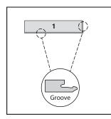
Start by positioning the first panel with the groove sides pointing away from the start walls.
