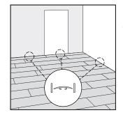
Provide expansion joints between different rooms or in large rooms. Check the supplier's guidelines for details.
