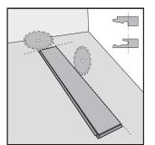
Remove the click profile on every side directly next to the wall to ensure the required expansion gap.
