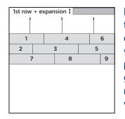
Move the rows closer to the wall, leaving a distance equal to the width of the start row plus the expansion gaps. Ensure the start row is at least 5 cm wide.
