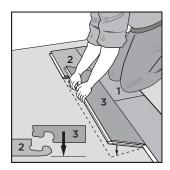
Engage the short side of panel 3 by pushing down. Ensure both panels are connected, push down along the joints of the panel.
