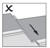
Do not lift up the side of the panel, angle down the edges of the panel, or shift the panels horizontally to disconnect the short sides. Doing so might damage the profile.
