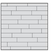
Complete the final row of the room by angling and dropping down the end row as calculated in the beginning.
