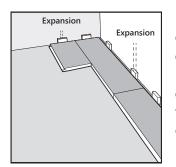
Place the spacers to ensure the correct expansion gap. For the correct expansion gaps, check the supplier installation guidelines.
