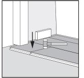
Drop down the short side and slide the panel towards the installed panels. Use a tapping block to hammer the long side in a few taps. Hammer down to fully connect the short side.
