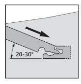
Place the tongue of the long side of panel 2 into the groove of the long side of panel 1 at 20-30° and angle down.
