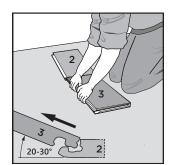
Angle up the end of the panel to angle out the short side.
