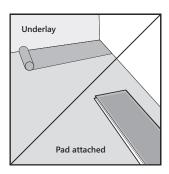
If there is no pad attached to the panels, roll out the underlay in the same direction of the floor.
