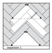
Mark the dimensions on the pre-build panels and cut to size.
