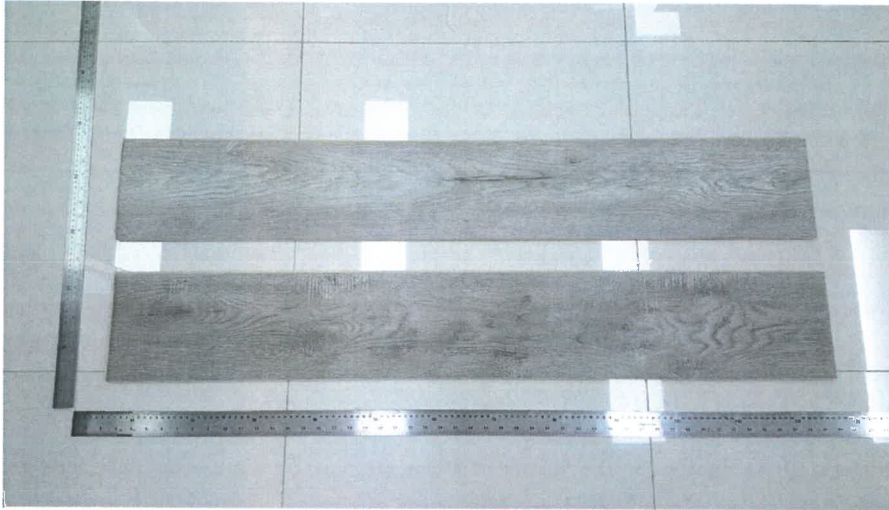
Photo 1. Tested sample – Wood Plastic Composite Flooring
